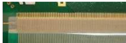
Ribbon cable to PCB connection - close up
