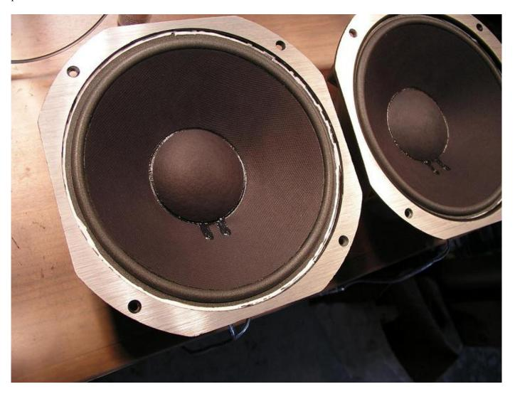
Now, its time to put the hard rubber ring into the basket edge. Run a thin bead of glue around the basket (see previous picture) – let dry a bit.
