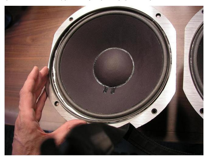
The two completed baskets, hooked-up and running the 30Hz test tone for the entire drying cycle. This is what the drying phase looks like. It's a bit boring, but oh-so-important. Keep that 30Hz tone playing constantly - it ensures the voice-coil is centered, and allows you to hear if things need adjusting. Check on them periodically, but go find something else to do
