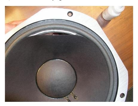
View of the surround and cone edge, with the wet glue. Looking good. The glue dries clear, so it looks even better when dried. Periodically, keep working around the cone edge, one finger behind, one if front, gently pushing the surround and edge together.
